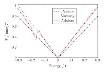
FIG. 3. (Color online) The transmission as a function of energy for pristine graphene (dashed), vacancy (red), and adatom (blue). The impurity is in between probes, which are separated by  $\sim$ 50 nm along the armchair direction. The dots denote a similar calculation using the SPA expression Eq. (13). The parameters for the adatom are chosen as in Ref. [56] as  $\epsilon_{\alpha} = -0.185|t|$  and  $t_{\alpha} = 0.37|t|$ .
