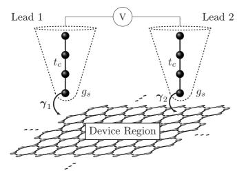
FIG. 1. Setup sketch including the leads modeled as onedimensional chains with a hopping  $t_c$  between the sites. The surface Green's functions  $g_s$  are indicated together with the coupling  $\gamma^{1/2}$ between the lead and the graphene sample.
