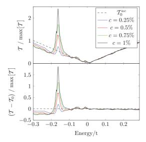
FIG. 5. (Color online) (a) Configuration-averaged transmission as a function of energy. (b) The difference between the averaged transmission and the pristine transmission. We place impurities in a  $50 \times 85$  nm square around the probes The unequal sides are chosen to take into account the probe separation direction. The curves are made from averaging  $2 \times 10^4$  configurations.
